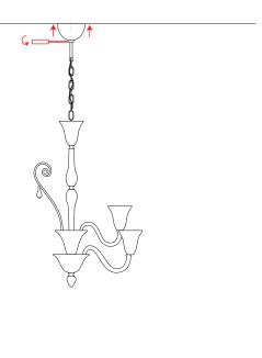
**STEP 5**Raise fondino and secure in place using finial components. Attach candle sleeve, cup and bulb.
