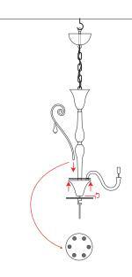
Insert glass elements into top tier fondino plate. Raise upper fondino to cover and secure beneath.
