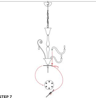
Install arms into lower fondino plate making electrical connections using 'click' connectors and securing beneath the plate.
