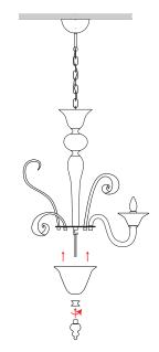
**STEP 7** Raise fondino and metal liner into position and secure using finial beneath.
