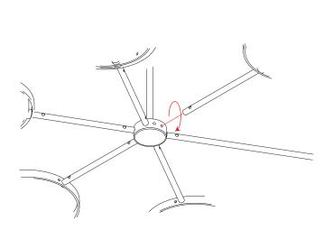
**STEP 4**Attach arms into each drum spacer and secure with hex nuts.
