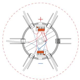
CONNECT ELECTRICAL CABLES AFTER STEMS WERE TIGHTENED
