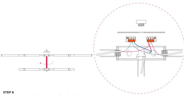
Attach lower tier to the drumspacer. Pass electrical cable through the hickey and connect electrical cables.
