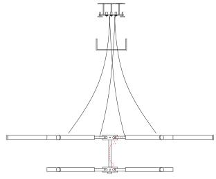
\*Pass electrical cables on the bottom tier through vertical stem and the stems on the top tiers.
