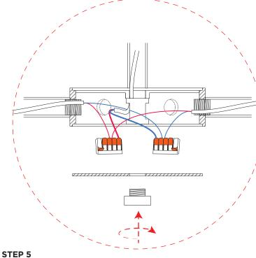
Close the fascia plate using the endcap. Screw the endcap into the hickey to secure.
