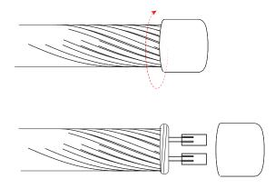
**STEP C TROUBLE SHOOTING - ELECTRICAL FAULTS**Remove the cap and check electrical connection.
