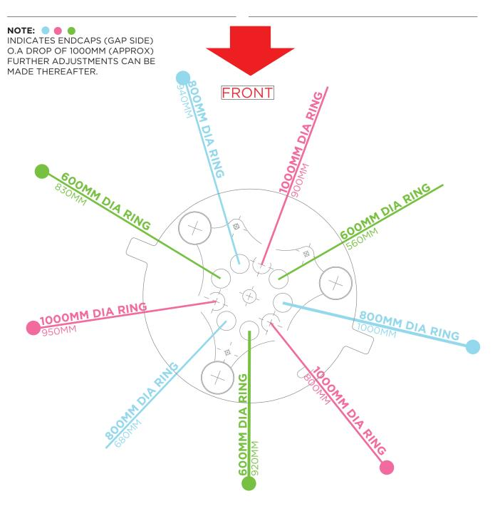
\*ENSURE ANY ELECTRICAL WORK IS CARRIED OUT BY A QUALIFIED ELECTRICIAN\* Illustration shows the view looking up at the ceiling plate.
