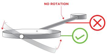
LOOSEN RING ANTICLOCKWISE INTO POSTION
