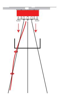
**STEP B TROUBLE SHOOTING - ELECTRICAL FAULTS**Lower ceiling canopy. Check/test connections.
